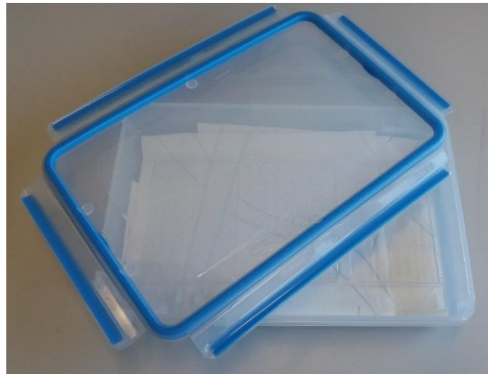
Fig. 3: Exemplary storage box with paper towel that can hold 3 Multiwell-MEA plates.
