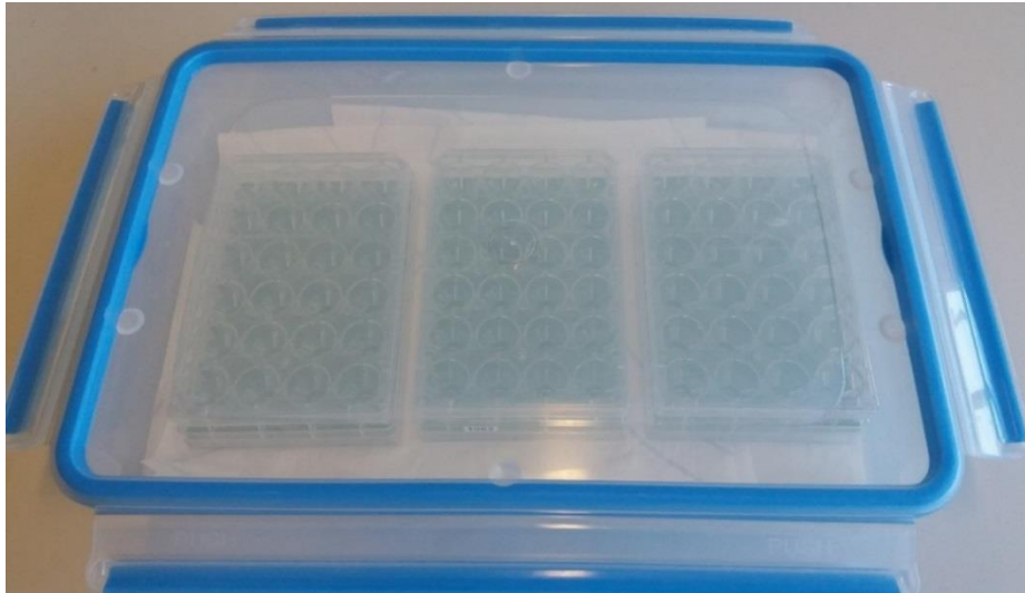
Fig. 6: Exemplary storage box with moistened paper towel, holding 3 Multiwell-MEA plates.
