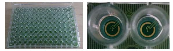
*Fig. 3: 96-well Multiwell plate. Left: Overview, right: Microscopic view into two wells. Note the three electrodes in the center of the well and the circular reference electrode. Cells ideally are only plated in the center without covering the reference electrode.*
