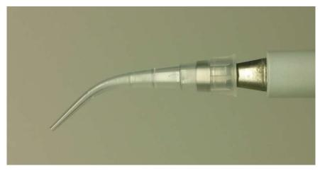
Fig. 1: Kinked 10 µl pipette. The tip was softened using a crème-brule burner and a forceps.
